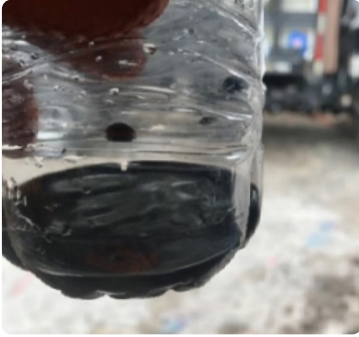
Figure 4 - Dark water pulled from a well and indicating that over purging or other well rehabilitation may be necessary.
