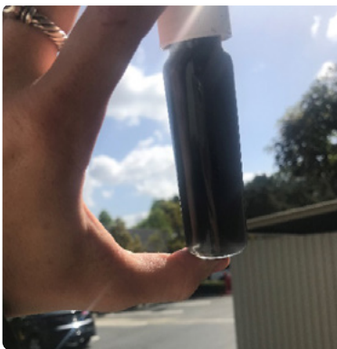
Figure 2 - Image of groundwater samples in a VOA bottle and exactly at 100 mg/L with some visible light coming through. Anything at this concentration or lower is safe to send to an analytical laboratory.
