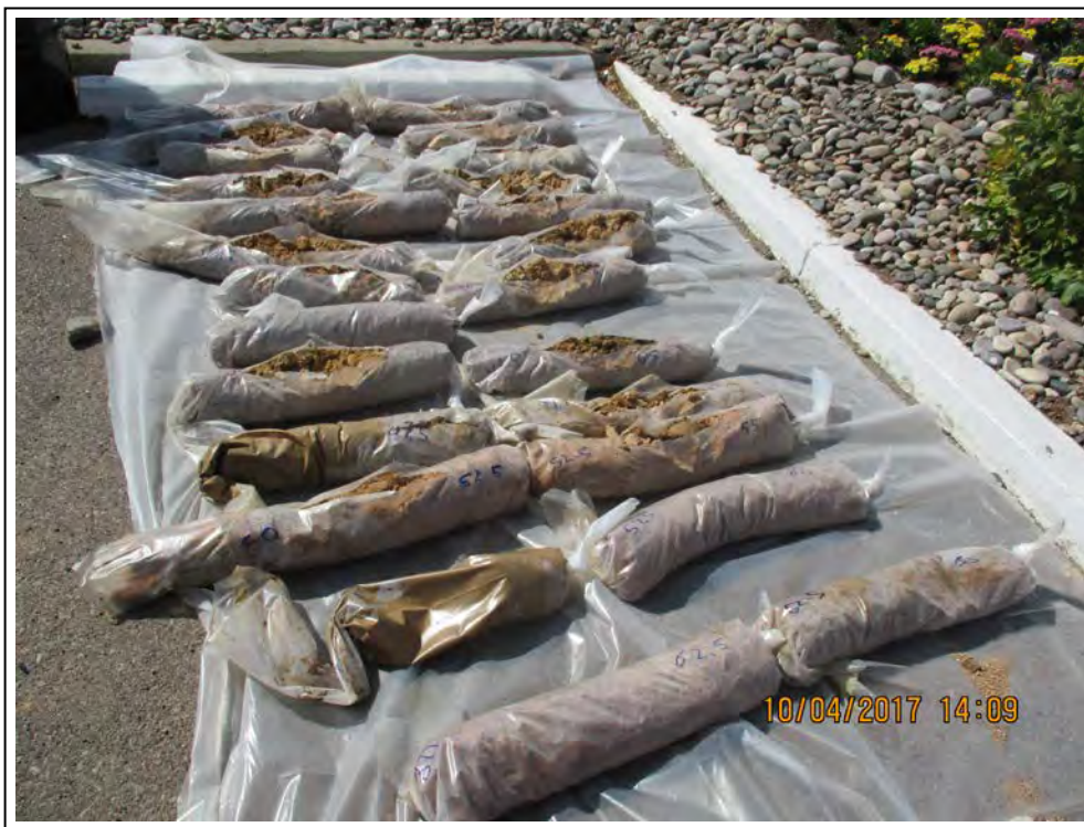
5. Sonic core samples from monitor well MW-16.
