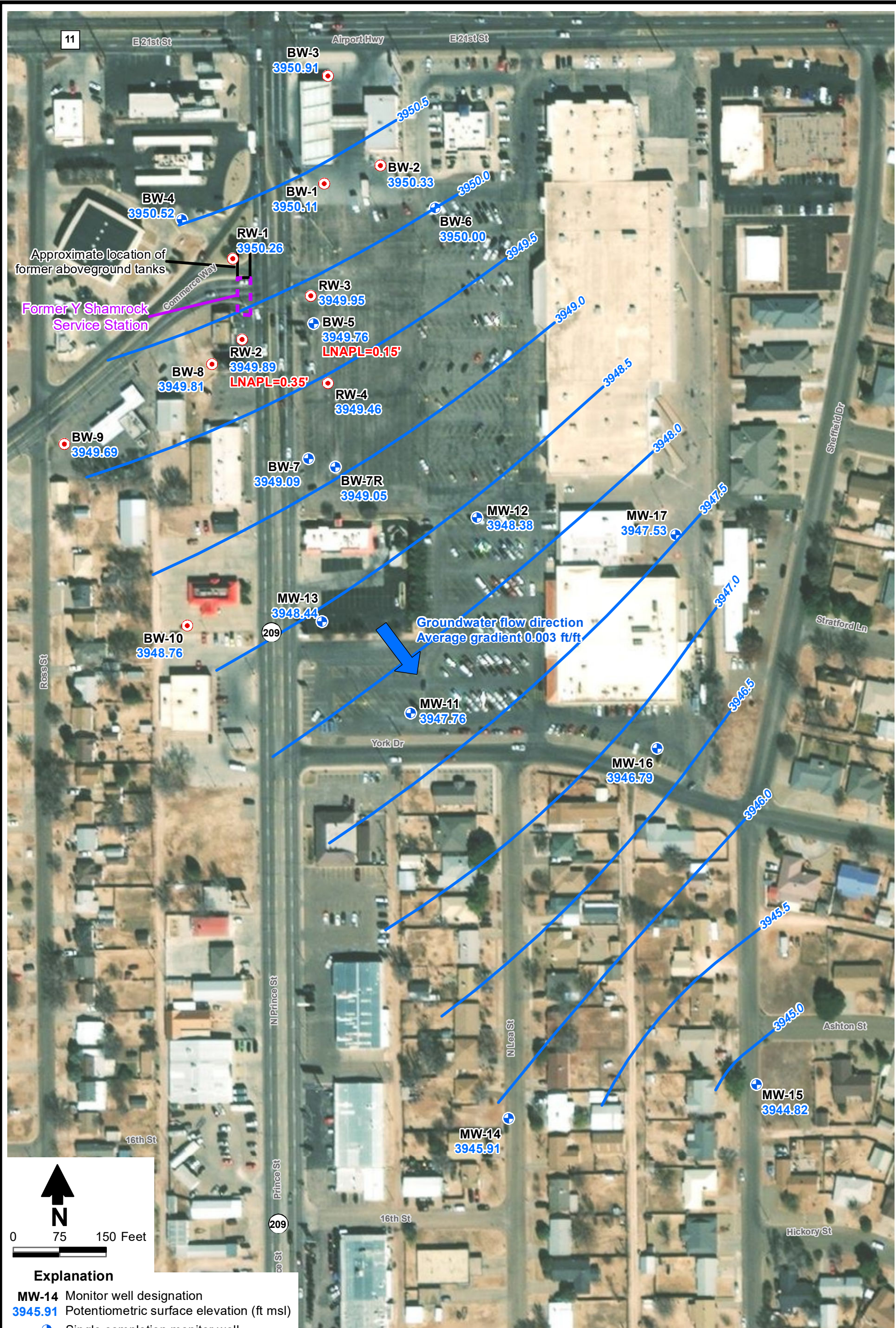
FORMER Y STATION STATE LEAD SITE CLOVIS, NEW MEXICO Potentiometric Surface Elevations March 19, 2021
