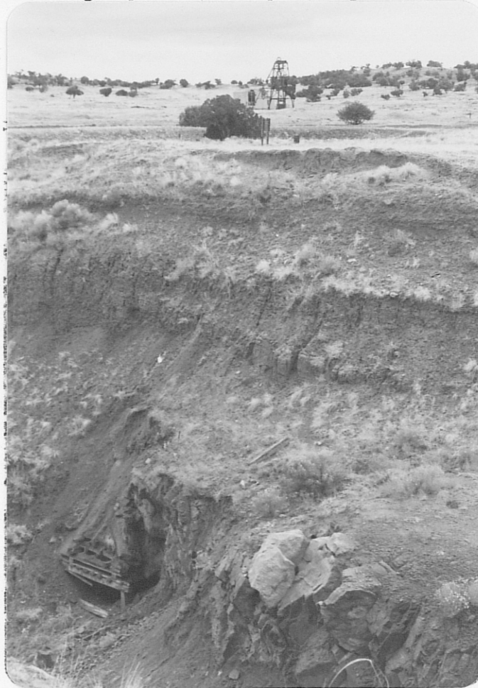
Photo (d) Looking northward into box cut with decline driven eastward at bottom. Close-up of decline is given on next page. Note section 25 head frame in background 1,000' away.
