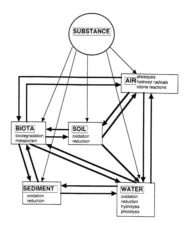
FIGURE A4.1 Diagram showing transport and transformation processes for substances in environmental compartments (after Calamari, 1994)
