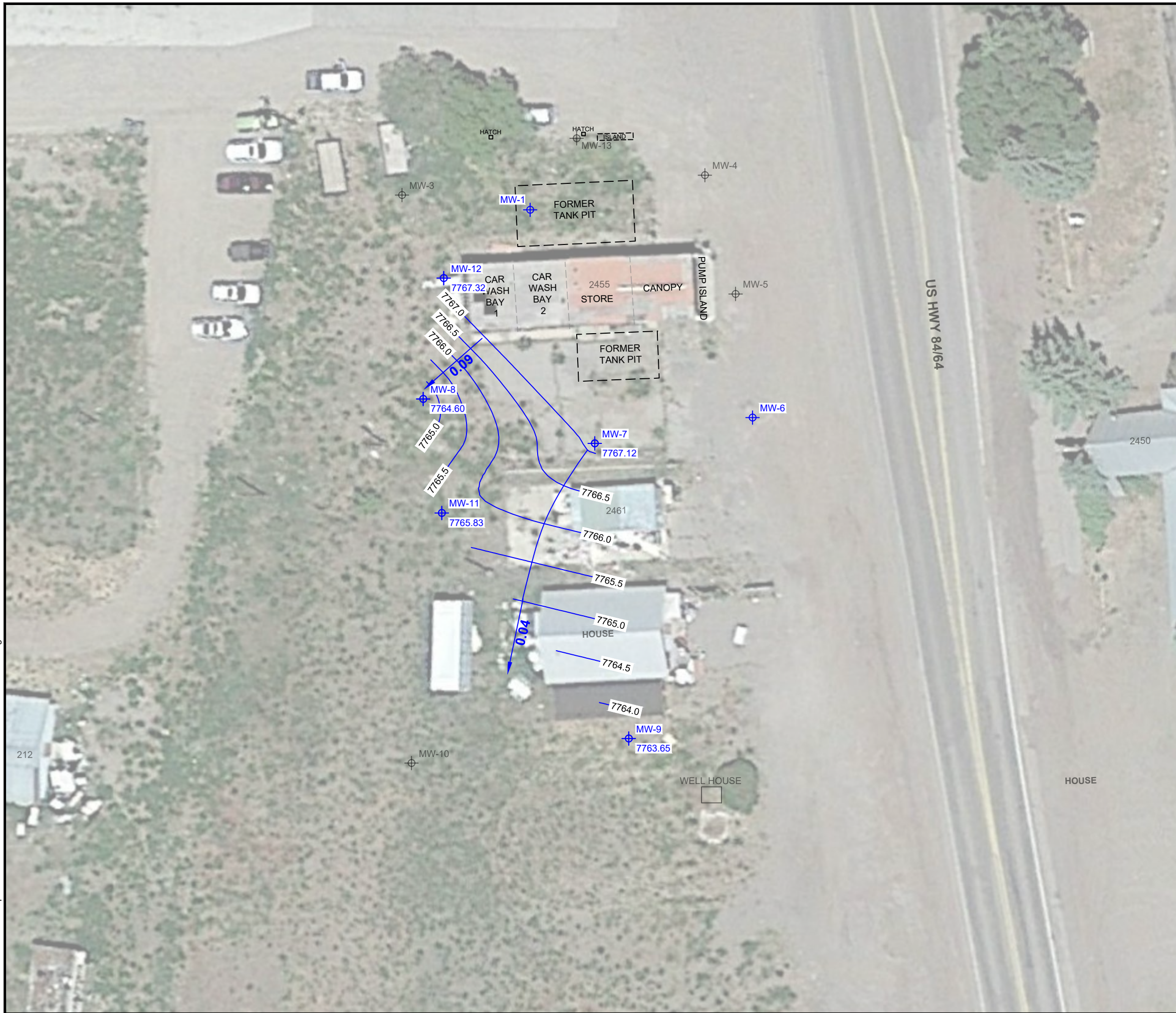
FIGURE 2 GROUNDWATER ELEVATION CONTOURS MARCH 31, 2022
