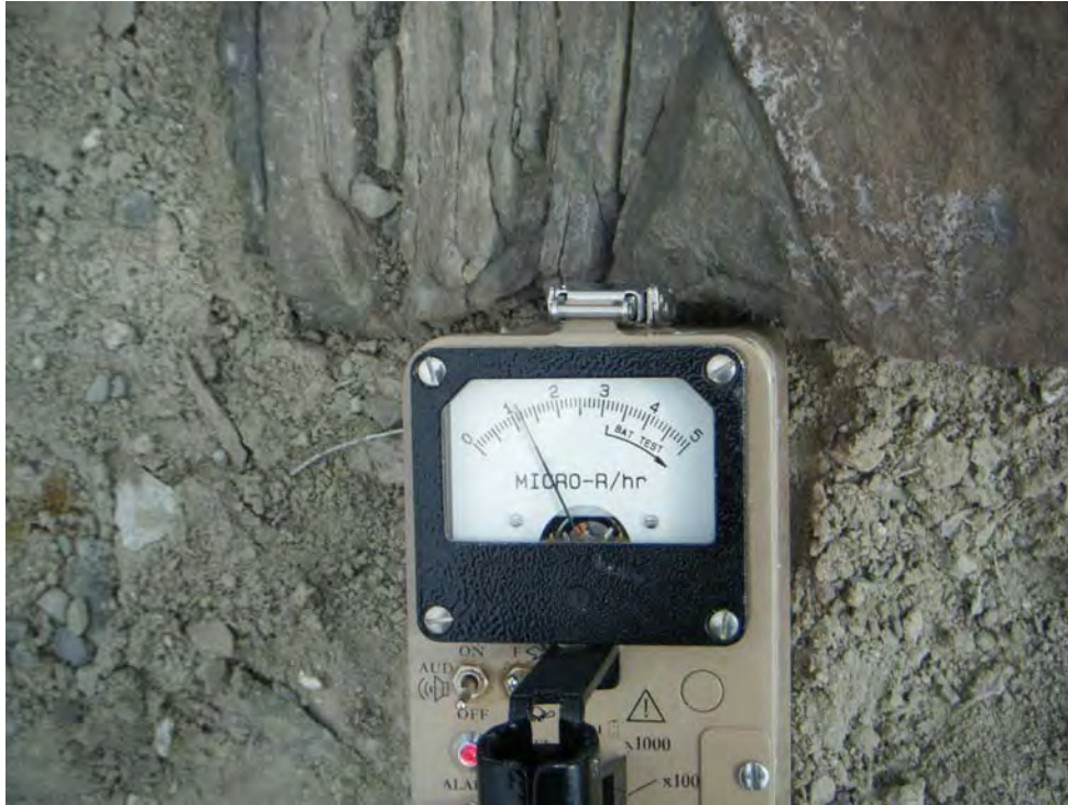
Photo 3-Looking at scintillometer reading on grey rock on PilePly-1 (Rad-2; 1200 \mu R/hr at contact).
