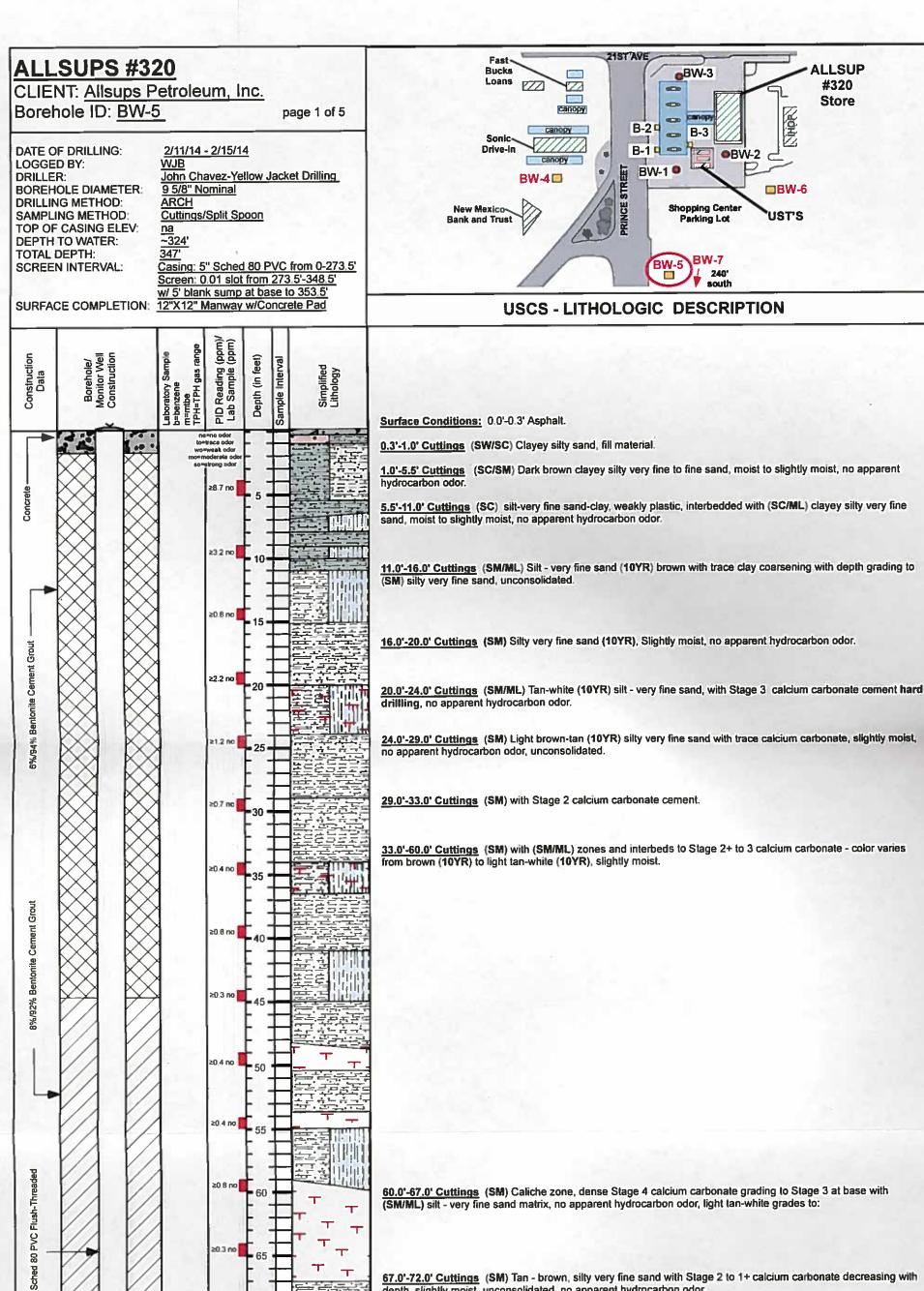
60.0'-67.0' Cuttings (SM) Caliche zone, dense Stage 4 calcium carbonate grading to Stage 3 at base with (SM/ML) silt - very fine sand matrix, no apparent hydrocarbon odor, light tan-white grades to:
