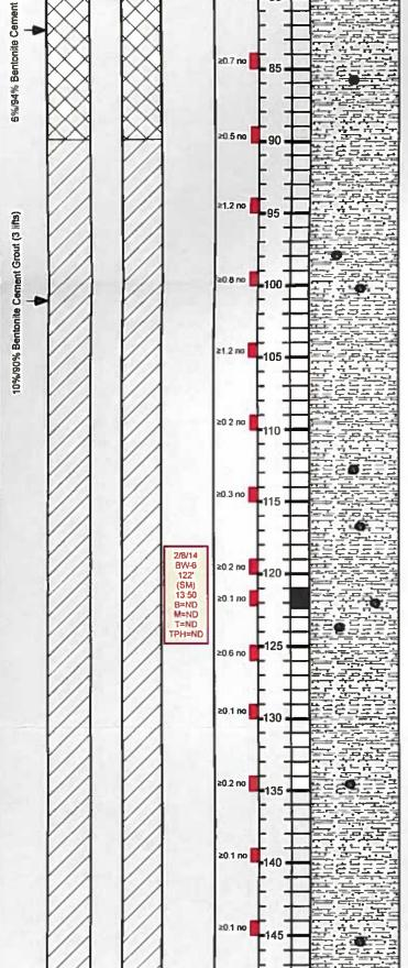
121.0'-122.5' Split Spoon 1.5' sample. (10YR) Silty very fine to fine sand, massive, weak calcium carbonate cement at base with localized calcium carbonate nodules, slightly moist, no apparent hydrocarbon odor.
