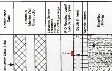
76.0'-130.0' Cuttings (SM) Silty very fine sand, unconsolidated, (10YR) brown, no apparent hydrocarbon odor, moist, occasional small calcium carbonate nodule, slightly moist to moist.
