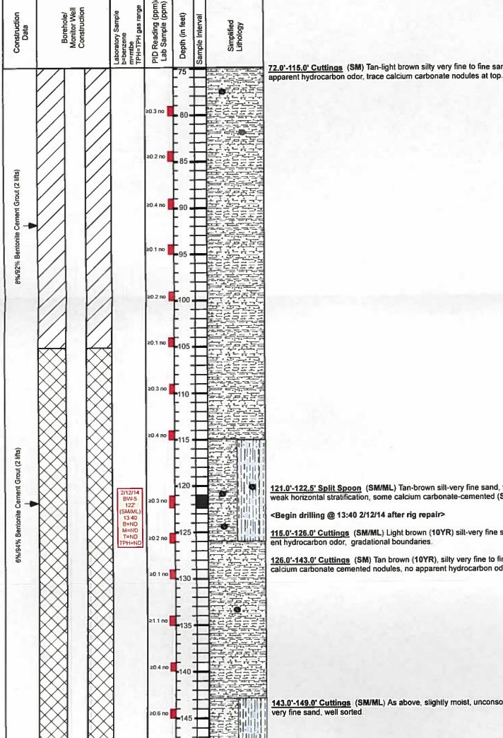
121.0'-122.5' Split Spoon (SM/ML) Tan-brown silt-very fine sand, finer grained than surrounding, some moisture, weak horizontal stratification, some calcium carbonate-cemented (SAS) sandstone nodules.
