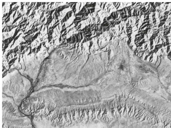
Fig. 4.11 Features associated with groundwater recharge in the sub-Himalayas; the thinning of streams towards downstream indicates influent seepage. (Landsat MSS4 image)
