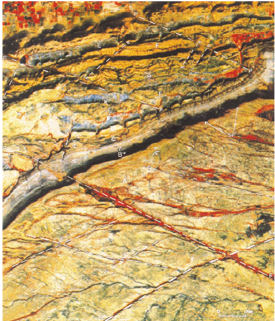
Fig. 4.15 Mapping of various types of fractures on IRS-1C LISS-III FCC of Cuddapah region, India. (Courtesy D.P. Rao, A. Bhattacharya and P.R. Reddy)
