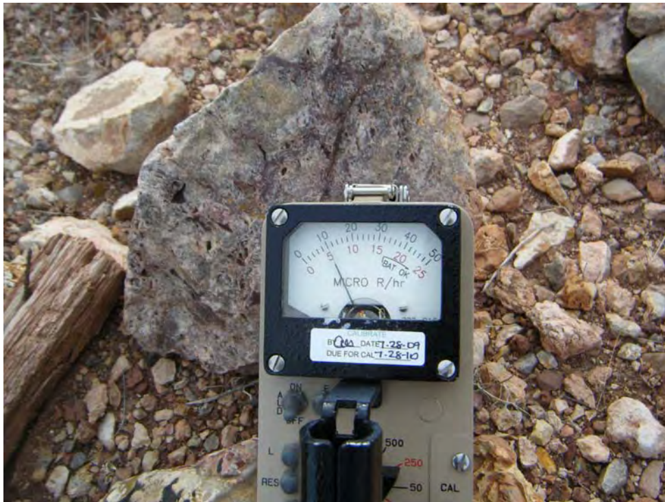
Photo 10 –Ludlum reading of 50 \mu R/hr (rad-3) on a rock on the west side of the bench (bench-1).
