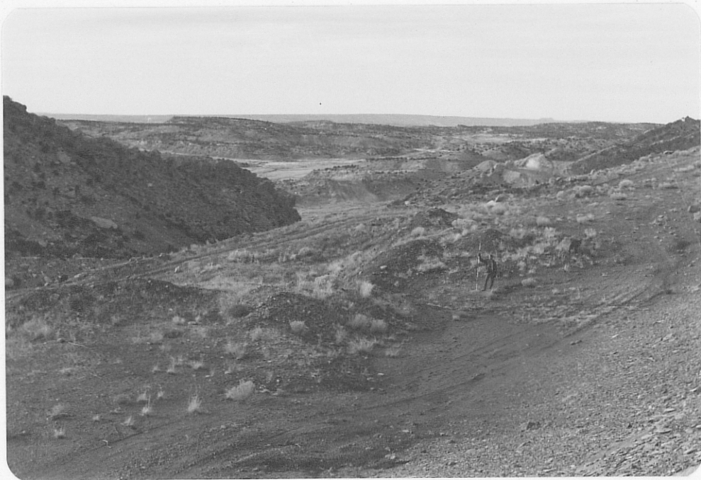
Photo (d) Looking north at stripped area. Bench has been constructed by open pit mining on dip slope in basal Dakota Sandstone.
