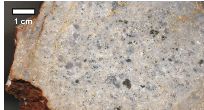
Sample Q10-18-02-4a, SE Straight Creek. Relatively intense QSP alteration. Dark clots are pyrite, white specks are plagioclase mostly replaced by fine sericite/illite.
