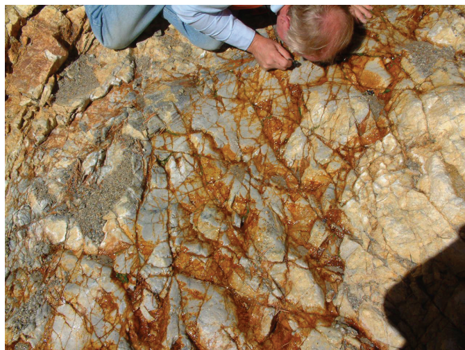
Figure 8. A, view of mine bench on the upper west wall of Molycorp open pit showing zone of QSP alteration crosscutting earlier propylitically altered andesite. QSP alteration is manifested on the surface by orange iron oxides and hydroxides generated by oxidation of pyrite. B, stockwork fractures in QSP-altered andesite, Straight Creek scar. Bright orange colors highlight acid waters flowing along fractures in stream channel. The volume of water gradually increased downstream from this locality, suggesting possible inflow of ground waters into the stream from shallow subsurface.
