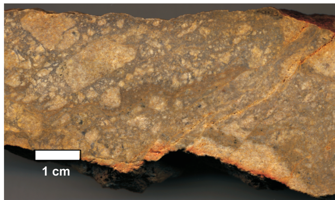
C. Sample Q02-22, from outcrop of breccia pipe on Molycorp mine site near ventilation air shaft. Hand sample photo shows hydrothermal breccia with clasts highly altered to pyrophyllite. Matrix contains a mix of pyrophyllite and silica.
