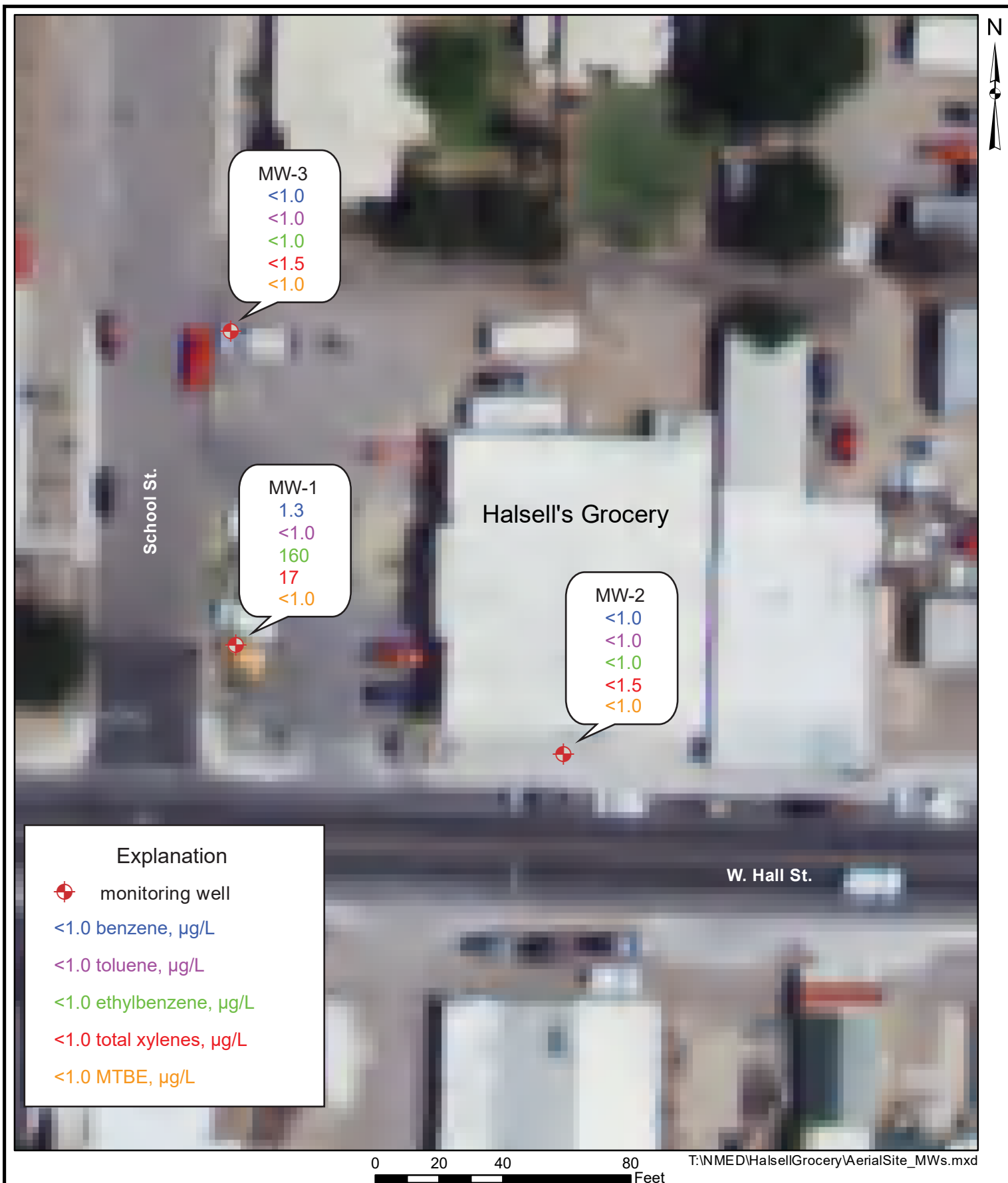
Figure 3. Site map showing BTEX and MTBE concentrations in monitoring wells, January 3, 2024, Halsell's Grocery site, Facility #6053, 112 School Street, Hatch, New Mexico.
