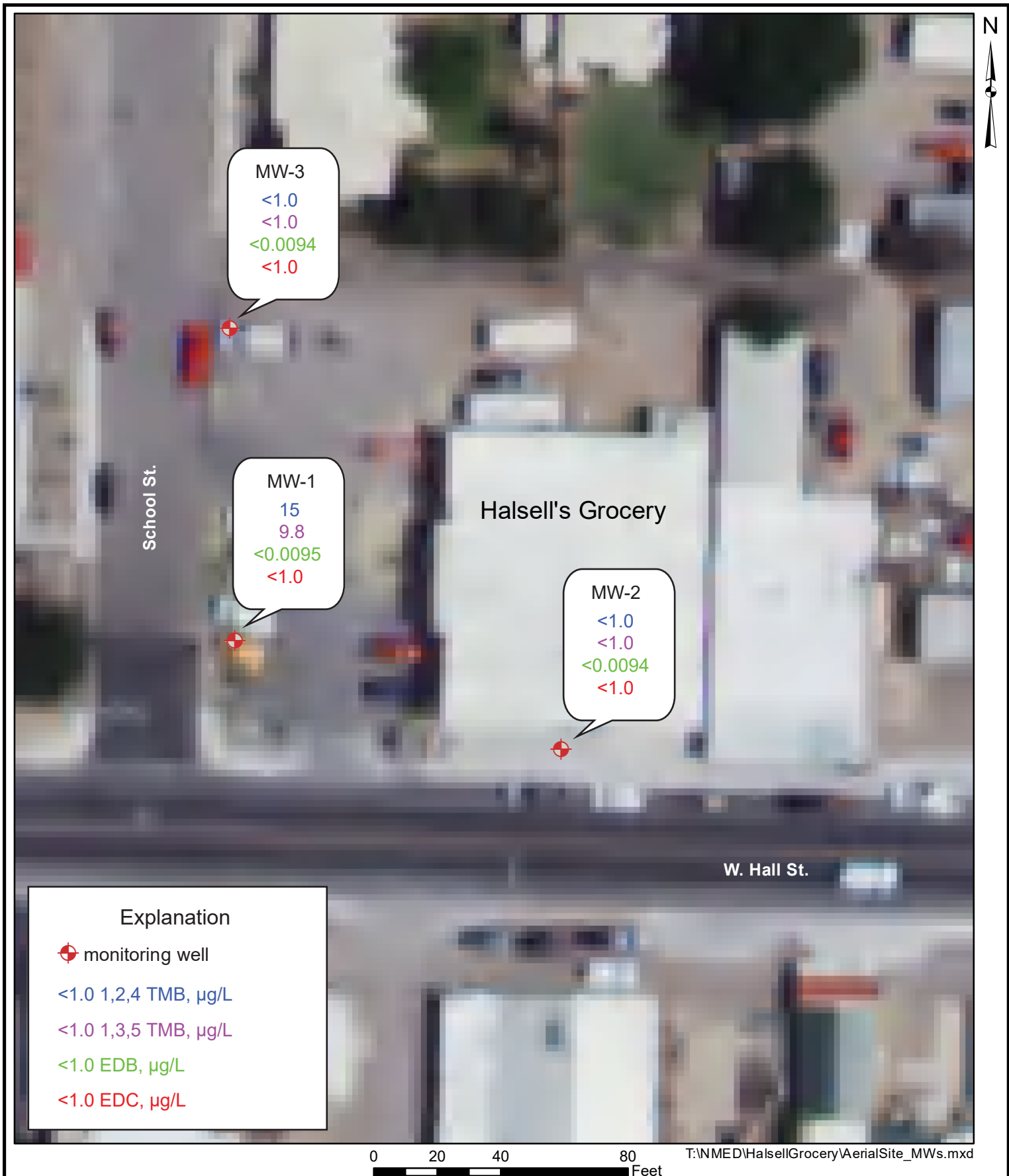
Figure 4. Site map showing 1,2,4-TMB, 1,3,5-TMB, EDB, and EDC concentrations in monitoring wells, January 3, 2024, Halsell's Grocery site, Facility #6053, 112 School Street, Hatch, New Mexico.
