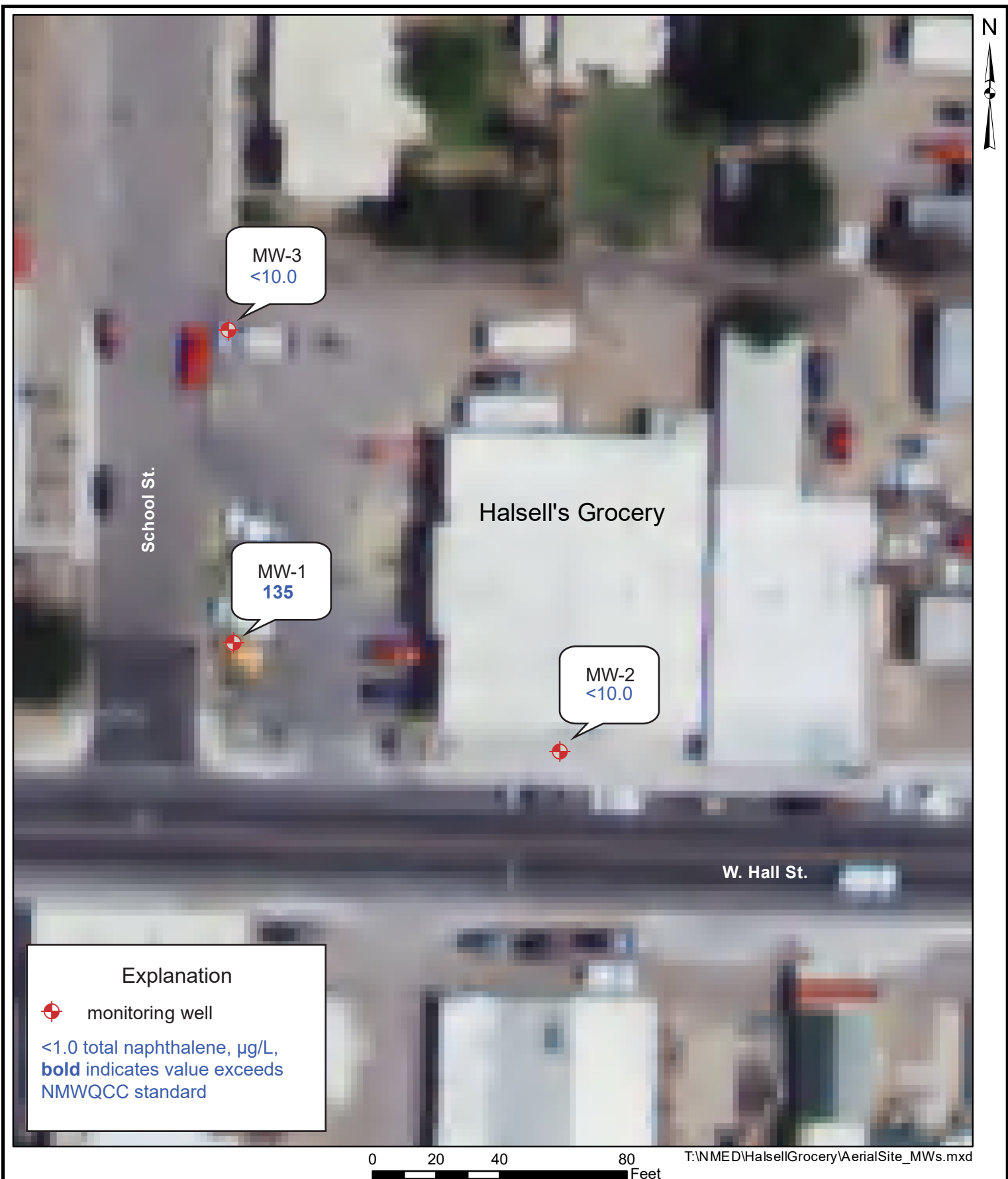
Figure 5. Site map showing total naphthalene concentrations in monitoring wells, January 3, 2024, Halsell's Grocery site, Facility #6053, 112 School Street, Hatch, New Mexico.
