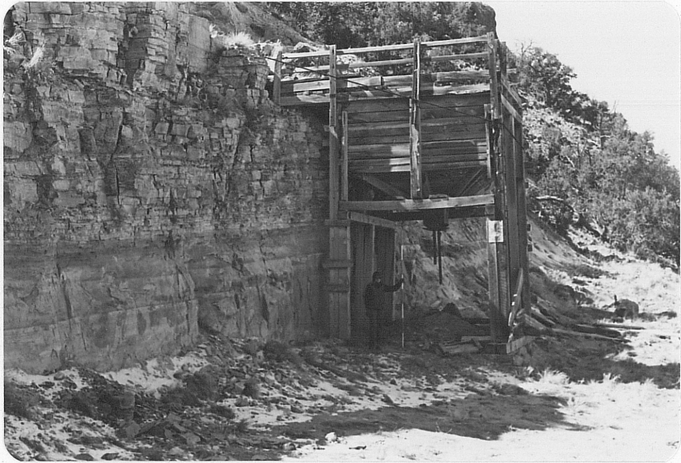
Photo (a) Looking westward at Lone Pine 3 load out facility; note Entrada-Todilto contact at left. Adits are at level of uppermost timbering.
