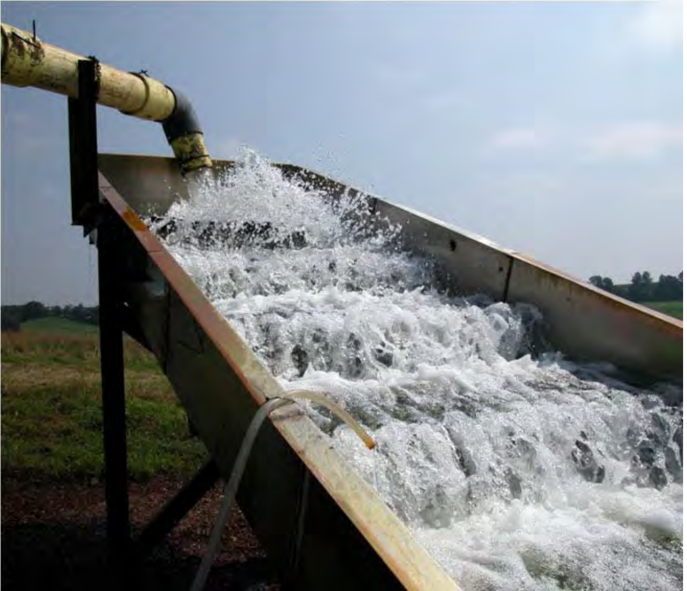
Photo 1. A 25° gravity-based cascading aeration flume (photo courtesy of Mike Kaufman, Chemstream, Inc.)
