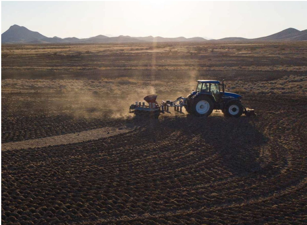
Figure 20. Agricultural tractor with keyline plow, imprinter and seeder. Treatment results in a loosened soil surface with waffle-like texture that captures seed, litter, and rainwater. Photo by Esha Chiochio.
