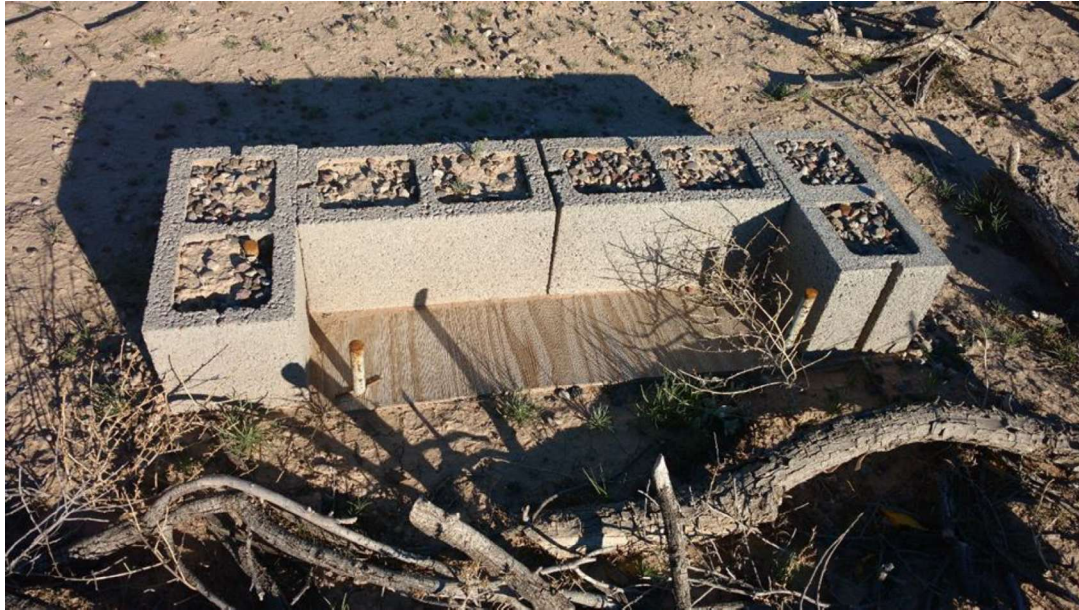
Figure 12. A sediment trap installed on a treatment with pecan branch mulch shows no accumulation of sediment.
