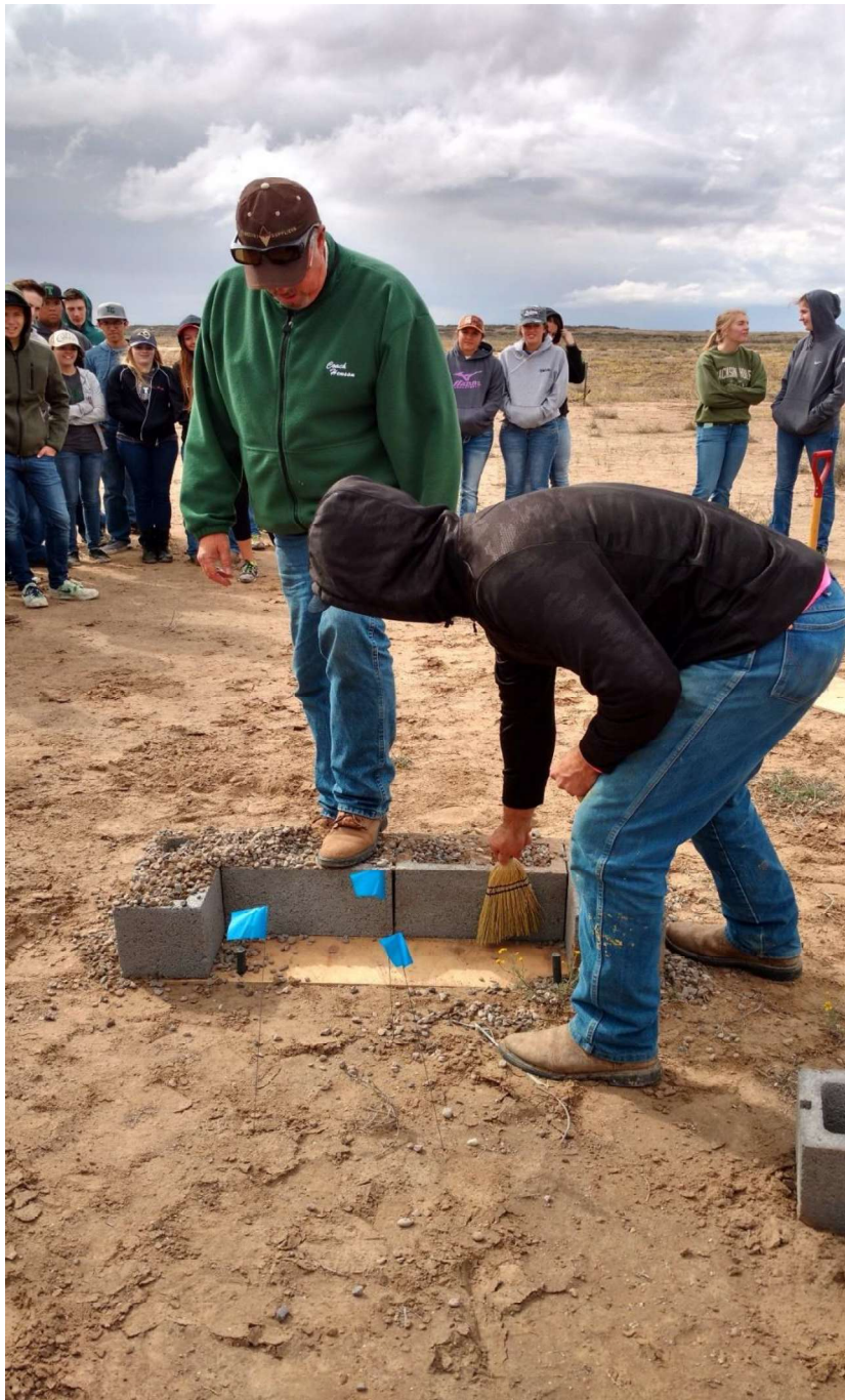
Figure 11. The anchored cinder blocks are filled with pea gravel to further secure the contraption. During monitoring the plywood floor is swept clean of debris with a whisk broom and dust pan. This debris is the sample which is taken back to the lab for weighing and laboratory analyses. The designer of the sediment trap, Dave Henson, is shown in the green sweatshirt.
