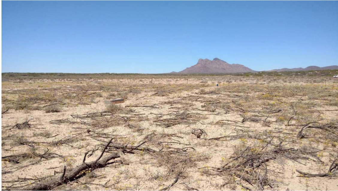
Figure 7. Pecan branch and gravel mulch were applied to a native grass seed plot. The view looks north toward a fence line. The bare control plots are located on the north side of the fence. Sediment traps were staged to capture surface water flow coming from north to south and from west to east. Note: the sediment trap at left center in the photo is sitting just outside of the plot. It was relocated to within plot.
