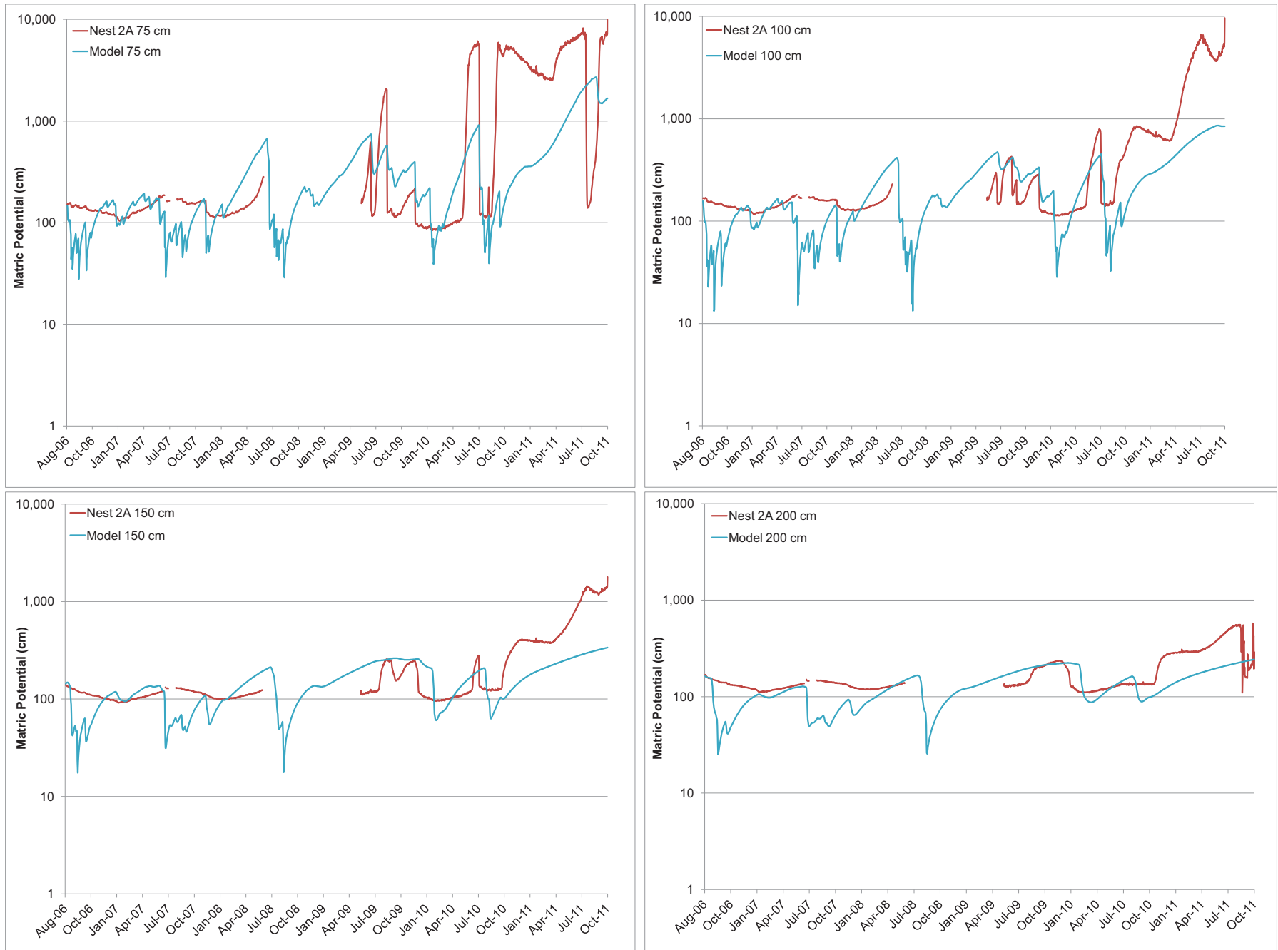
Figure 5: Simulated and Measured Matrix Potentials Top Surface 3-ft Cover Treatment
