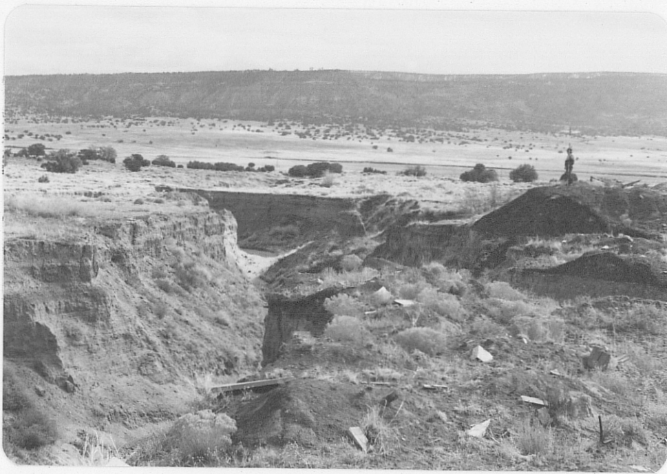
Photo C Looking southeastward down drainage that skirts main shaft area; mine waste perched on edge of bank has gamma valves of 10X background.
