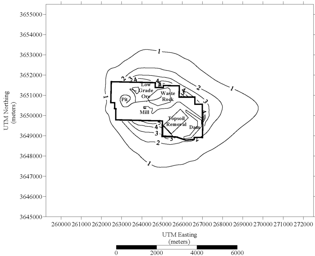
Figure 31: Isopleth of Copper Flat Mine's TSP Refined Model Results Copper Flat Mine Sources and Significant Neighboring Sources Annual Average ( \mu\text{g}/\text{m}^3 )
