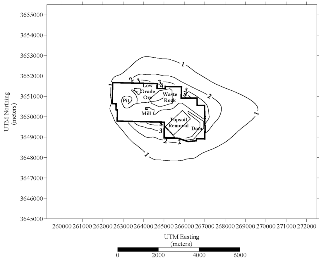
Figure 40: Isopleth of NMCC's Copper Flat Mine PM 10 Class II Increment Model Results NMCC's Copper Flat Mine plus Increment Consuming Neighboring Sources Annual Average (µg/m 3 )
