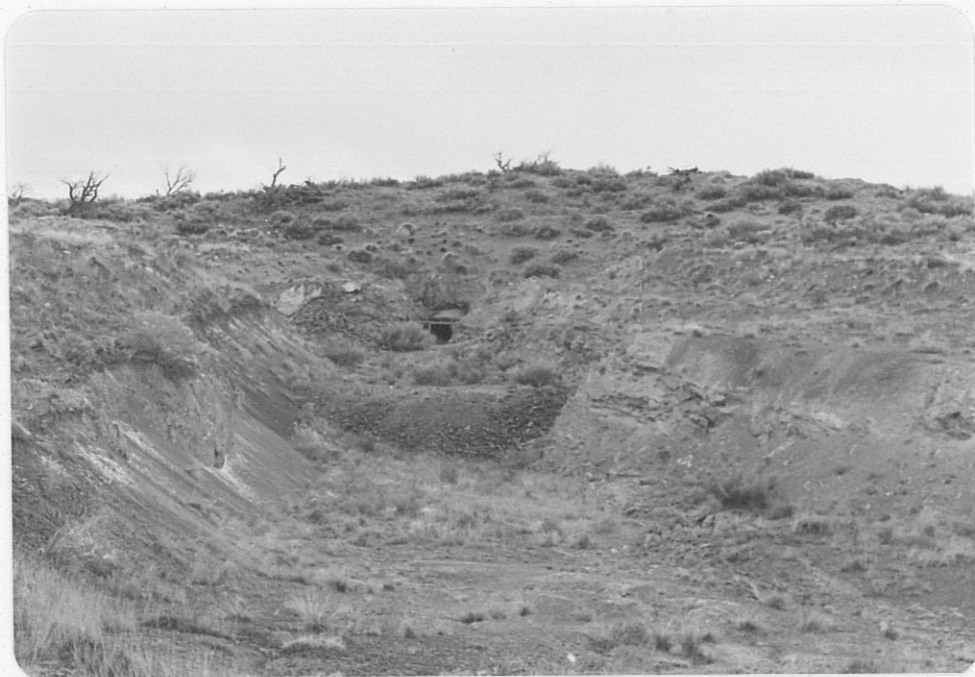
Photo (i) Looking westward inot west trending cut with adit at west end; cut is 325' long, up to 50' wide. Scintillometer response is strong, 1000 cps.
