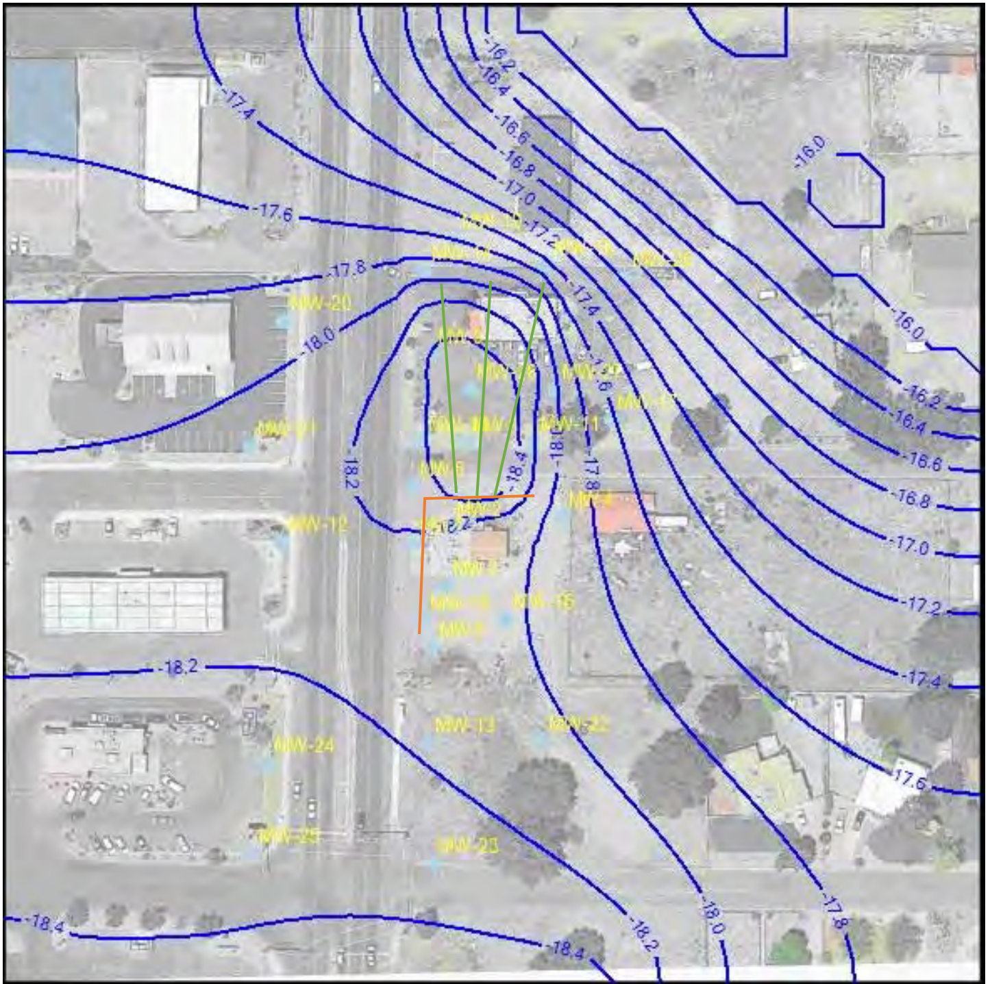
9. Horizontal Drains 2.2 to 2.5 feet below water table – 7.2 gpm
