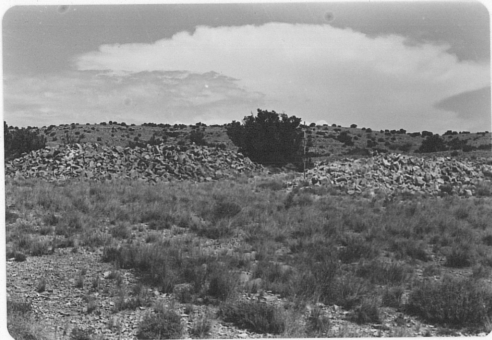
Photo (b) Looking northeastward at mine dump or low grade ore piles; left one is composed of Entrada sandstone, right one Todilto limestone; each is about 4' high.
