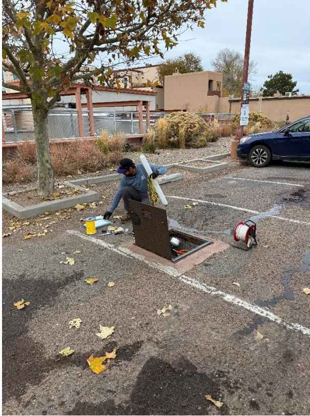
Photograph No. 1 Description: Groundwater sampling at SVE-6.
