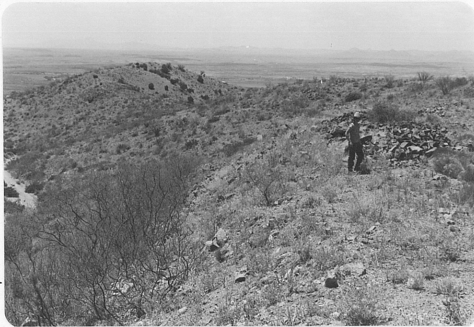
Photo (c) Looking westward at small tailings pile and lip of bench cut directly out front of adit in photo (b). Note small drainage at far left.
