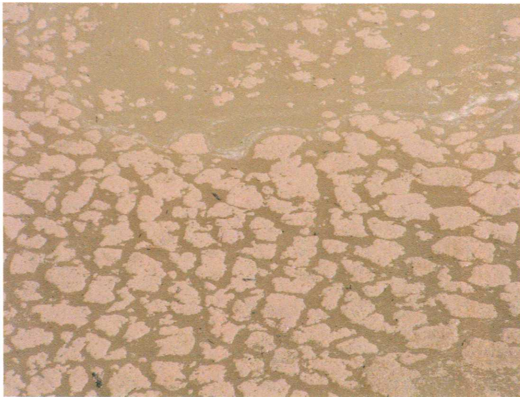
Photo 18. Close-up of groundwater and NAPL that was removed from the excavated area.
