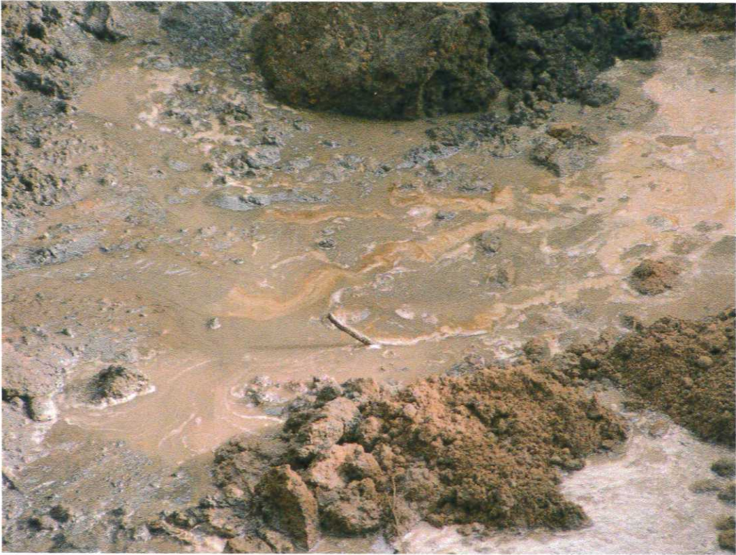
Photo 9. Groundwater with a thin layer of NAPL seeping out of saturated soil.
