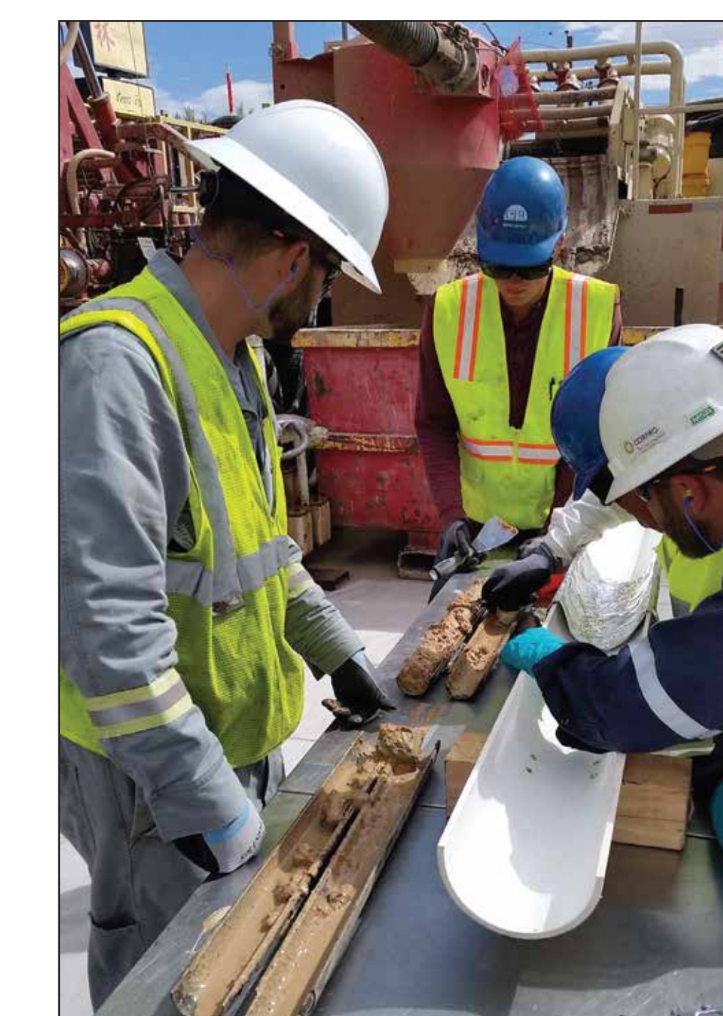
Looking at split spoon for lithologic description
