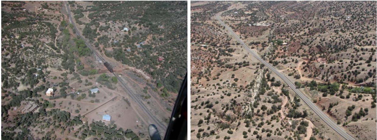
**Figure A.11.** (Bottom Left): The former Atchison, Topeka, and Santa Fe Railroad bisects the Galisteo Creek floodplain, creating separated riparian areas on both sides of the railroad grade. Only one side remains wet due to the Galisteo Creek; the other side has dried up since rail line construction in 1880. **Figure A.12.** (Bottom Right): State Highway 14 cuts across geologic features and streams, wetlands and spring areas east of the Cerrillos Hills in the “Garden of the Gods” area.
