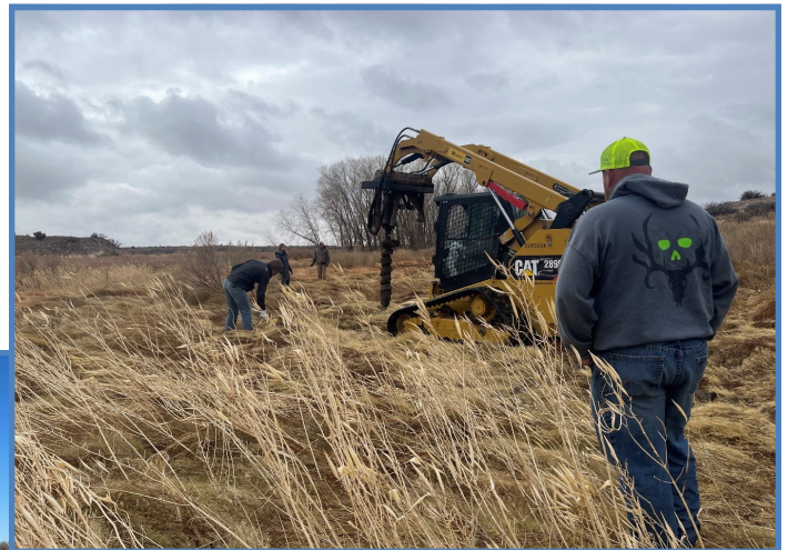
Photo above; Skid steer auguring holes for cottonwood poles.
