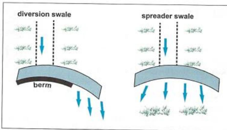
Figure 18. Contour Swales. (Diagram courtesy of.)
