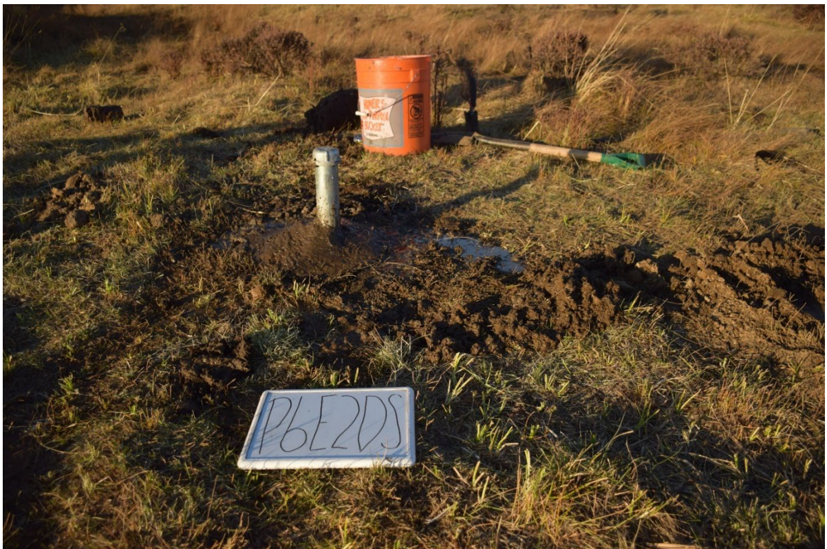
Figure 15. Completed piezometer P6E2DS in the East Drainage just up hill of FS 1910. Photo Emile Sawyer.
