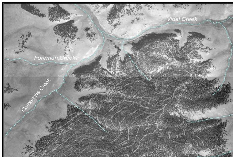
*Figure 9 Roads from jammer logging near the confluences of Comanche Creek with Forman and Vidal Creeks. DOQQs from the late 1990s courtesy of USFS Carson National Forest. The line across the middle of the picture is the join between two aerial photographs.*
