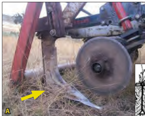
Figure 1.8A. The keyline plow uses a shank (yellow arrow) which creates space in the subsoil (Figure 1.8B). Figure 1.8C. The keyline plow is used in Keyline Design to make parallel furrows without inverting the soil surface, as shown in the photograph.
