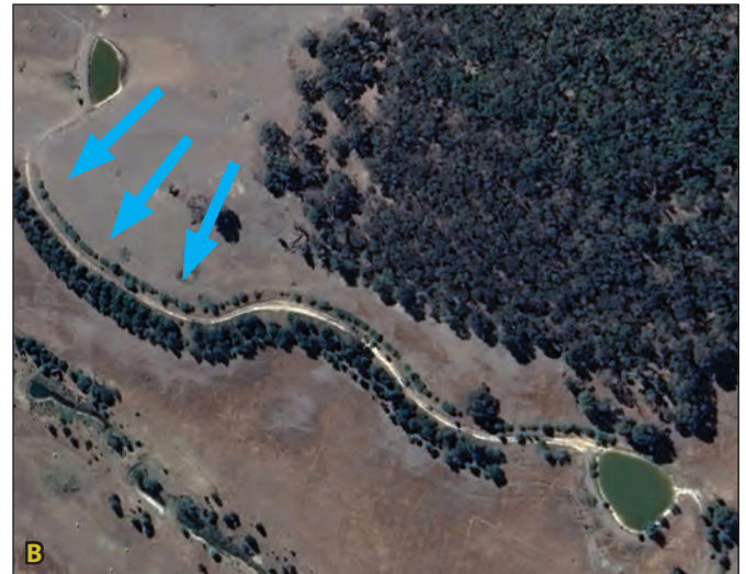
Figure 1.7A. Cross-section graphic shows a swale and berm with a hedgerow planted on the berm. Figure 1.7B. An aerial view of a dense hedgerow in conjunction with an on-contour swale and berm is shown at Taranaki Farm. Blue arrows show the direction of water flow down the hillside.
