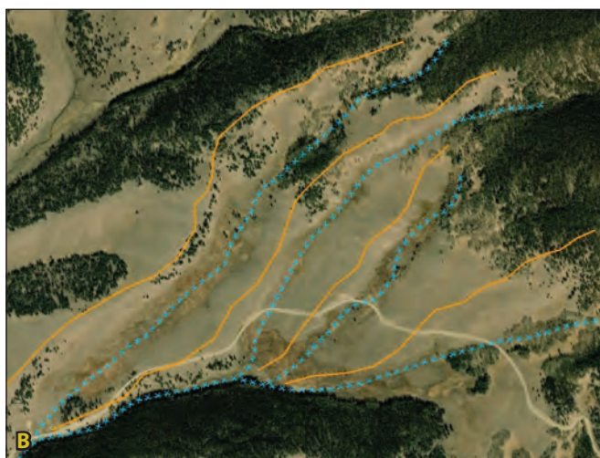
Figure 1.10A. In this aerial view of the Holman Creek Wetland Complex (bisected by Forest Service Road 1950), the white arrow points north. Figure 1.10B. Overlay on the same image of approximate ridge lines (orange) and wetland valley thalwegs (blue lines).
