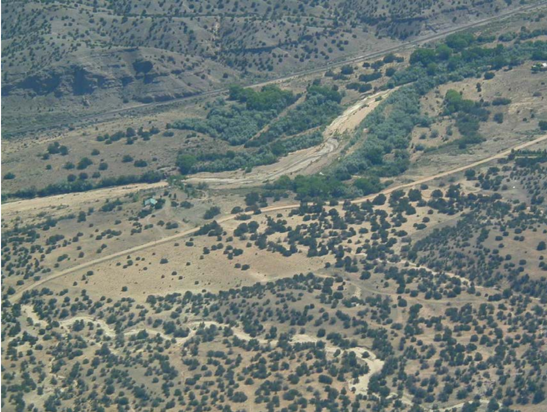
Figure 4. Aerial photograph of Galisteo Creek in the central part of the Galisteo Watershed. The photo shows riparian vegetation patterns that originate from levees constructed by the US Army Corps of Engineers between the 1930s and the 1950s to divert the Galisteo Creek away from the railroad tracks (top of photo). Induced meandering restoration techniques were used to recover stream hydrology, and restore overbank flooding and floodplain function within the confines created by locating railroad tracks adjacent to Galisteo Creek. All land shown in the picture is privately owned.
